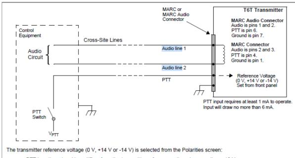
PTT is active when V<sub>PTT</sub> differs from the transmitter reference voltage by more than ±10 V
