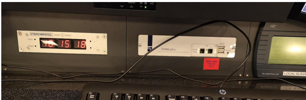
Figure 24: Gorgy clock and KVM switch on the Faceplate.
