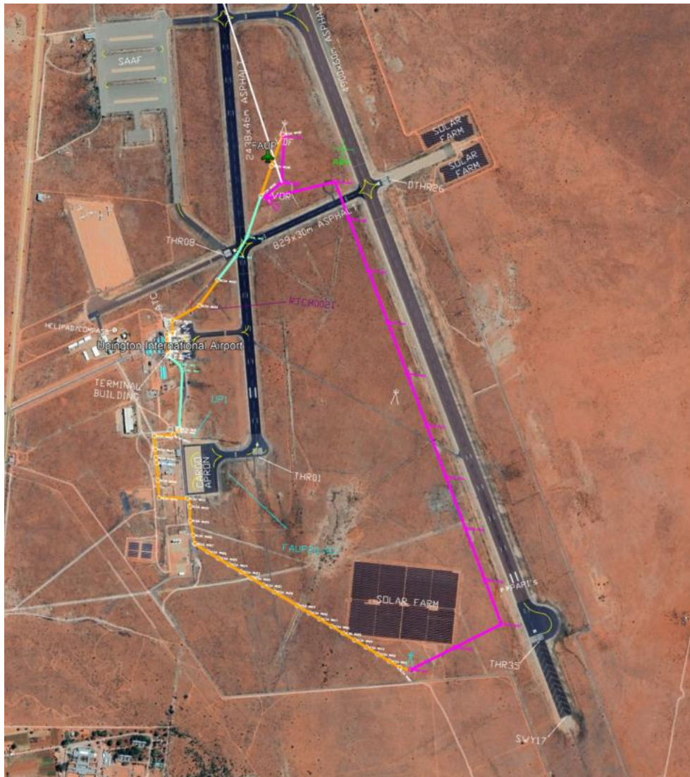
Figure 4: FAUP Fibre Route
